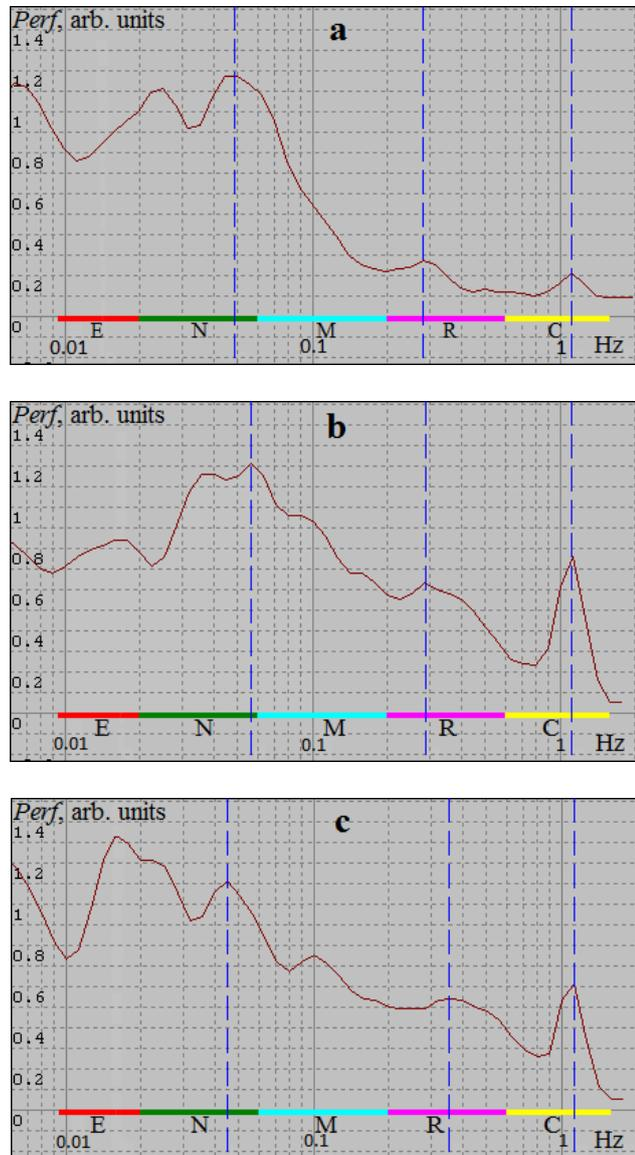
**Fig. 9.** Wavelet spectra of the base records of the l.d.f. (a), n.f.s. at 568 nm (b) and 808 nm (c) signals. Dotted lines show local maximums of the spectrum in the respective frequency ranges.
