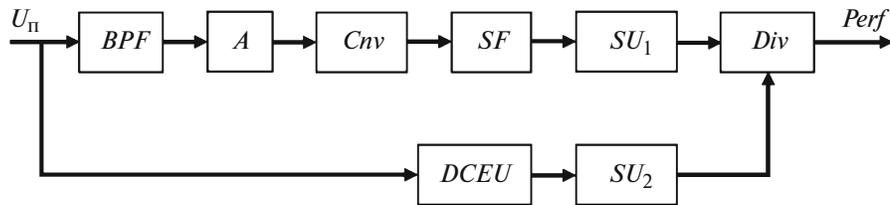
**Fig. 6.** The block diagram of the perfusion-index determination and indication unit: (*BPF*) bandpass filter, (*A*) amplifier, (*Cnv*) RMS-DC converter, (*SF*) smoothing filter, (*SU<sub>1</sub>*, *SU<sub>2</sub>*) squaring units, (*DCEU*) DC signal component extraction unit, and (*Div*) divider.
