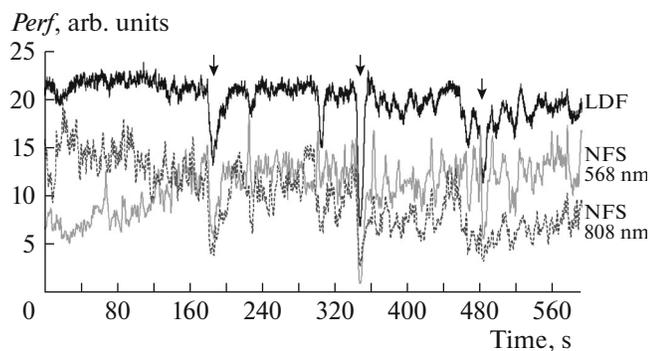
**Fig. 7.** The base records of the perfusion index *Perf* from the fingertips of the hand of the tested person that were obtained using the LDF and NFS methods. Arrows indicate the moments of involuntary sighs of the tested volunteer.
