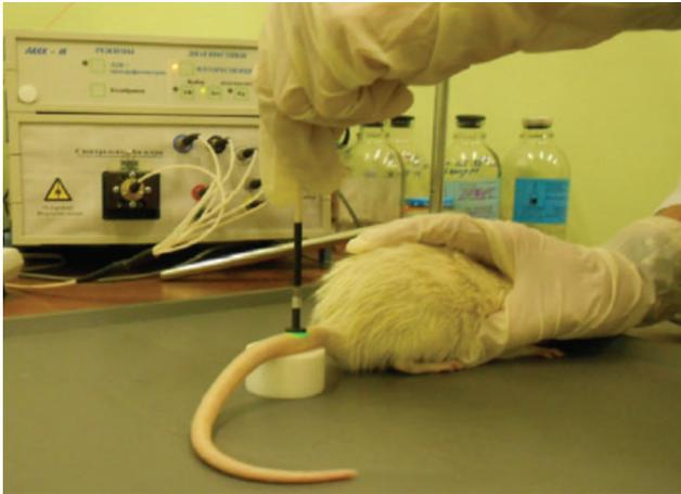
**Figure 8** The measuring procedure with the use of small animals and “LAKK-M” diagnostic system. Using the fiber-optical probe, the fluorescent spectrum is measured from a mouse tail.
